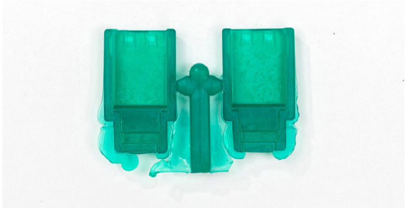
Flash caused by overfilling a mold.
